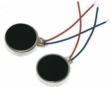
Haptic motors for vibrational output.
